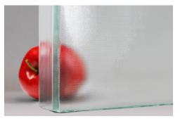
"filtered image" of the occupants and activities on the other side of the wall, simultaneously dividing and connecting people and spaces. The "fine mesh" channel glass texture also complements adjacent materials, including the aluminum foam cladding and fabric curtains.
